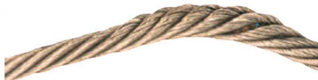
Figure D.4 - Extrusion de torons
